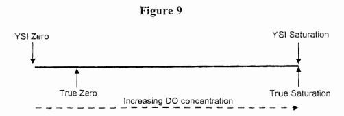
Figure 1 Relationship of YSI Model 55 DO probe readings to true DO readings
